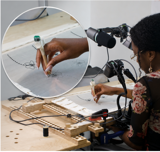
Figure 1: ANTLE 1 capture setup during a live tambour embroidery session. Overhead and underside cameras record stitch trajectory, fabric interaction, and embodied hand movement in real time. A sensor-integrated tambour tool captures fine-grained needle-motion dynamics used for segmentation and downstream co-creative coaching feedback.
