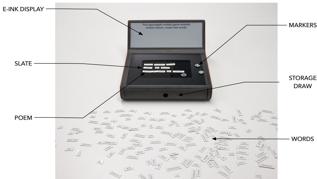
Figure 1: The Mimetic Poet machine, showing key elements of the device
