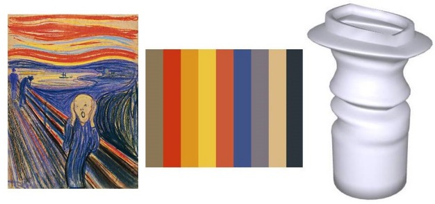
Figure 6: Depiction of the complete vase generation process using inspiration from one version of the famous Scream works by Edvard Munch.
