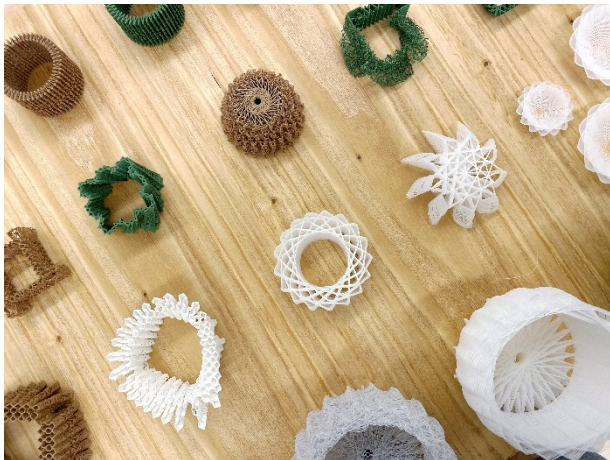
Figure 7: The top view of 3D printed objects with various layers of patterns and manipulated Z-height extrusion.
