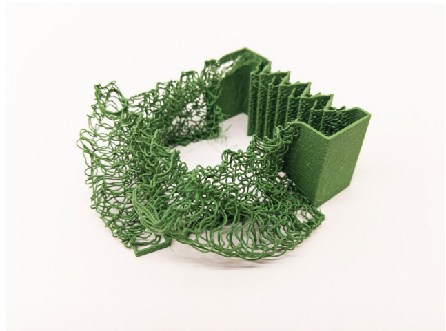
Figure 5: This model is composed of two different structures, loose and tight; the tight structure to solve the unraveling problem.
