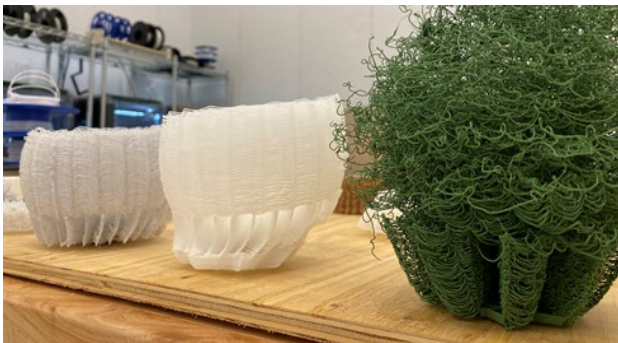
Figure 3: Low bed temperature made models not stick to the ground, so they moved and shifted while printing.
